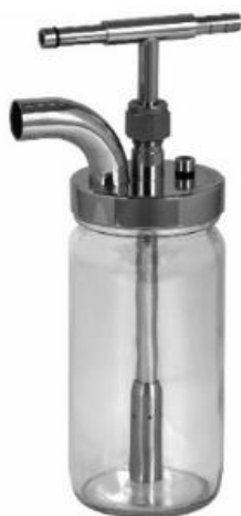
Figure 5. 6-Jet Collison nebulizer. BGI Industries made the Glass and 304 stainless steel construction.
