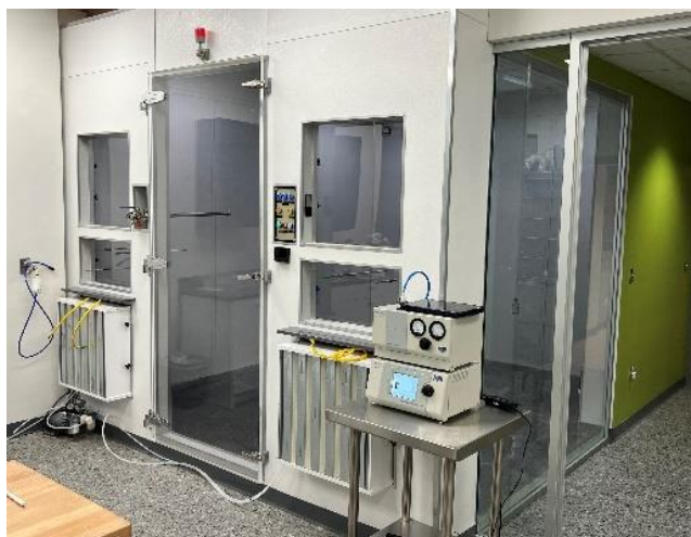
Figure 3: The 30 m 3 bioaerosol testing chamber at ARE Labs adheres to AHAM AC-5 standards and ASHRAE 241 criteria.
